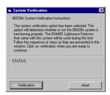
4. The System Verification procedure will start by performing an auto-bias routine. Ensure that a BNC 50 ohm load is connected to the Port 1 bias tee on the 8517B rear panel.
